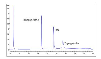
Figure 1. A test chromatogram of a Proteomix<sup>®</sup> RP-1000 column (5µm, 1000Å, 4.6 x 150 mm)
